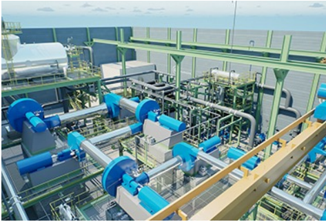
Visualization of the ComprivAP plant featuring an 11-stage compressor system from PILLER. © GIG Karasek
